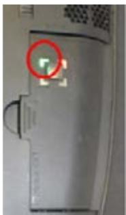
To check that the inflator is new and properly connected, take the In&box, put it on and insert in its housing. The inflator LED should switch to green.
