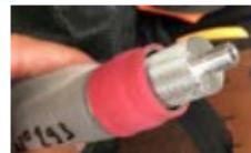
Check that the seal is positioned correctly and is not damaged.
